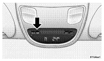
Compass Variance is the difference between magnetic north and geographic north. In some areas of the country, the difference between magnetic and geographic north is great enough to cause the compass to give false readings. If this occurs, the compass variance must be set according to the Compass Variance Map.
